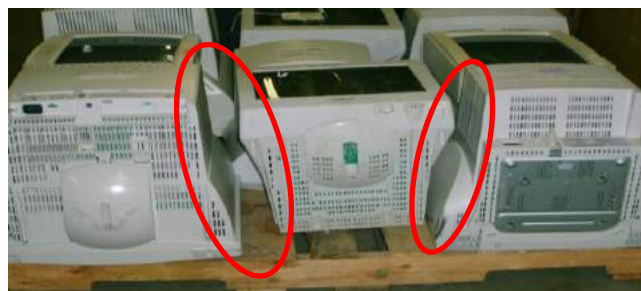
Monitors will normally fit together nicely when using the face up/face down pattern
