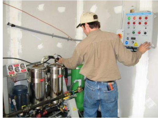
Blending used oil and heating fuel.
