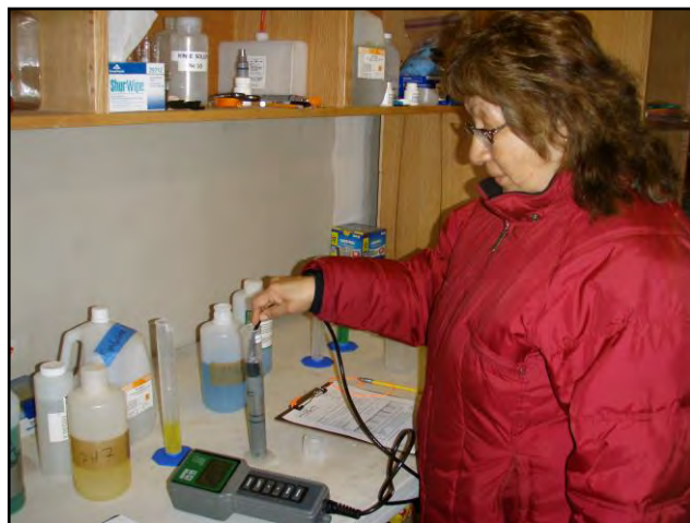
Hazel Lolnitz, Koyukuk Tribal Council, calibrates a YSI 63 during a water quality training in Fairbanks.
